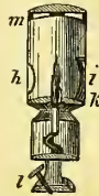
Lamp h , aperture with mica. h , diaphragm. i , screw for fixing lamp. § 2.
